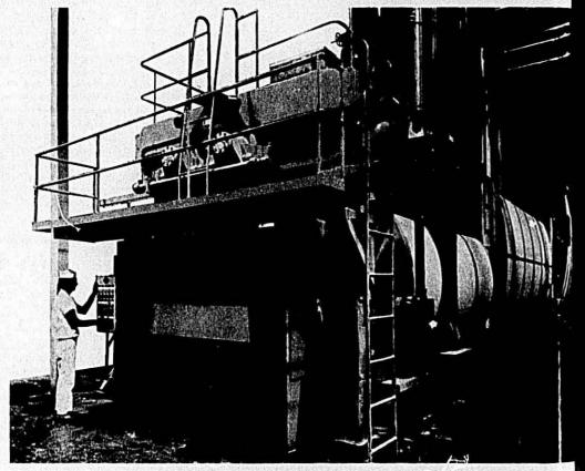
Long goods line with maximum capacity of 3000 lbs/hr. Line consists of Double Screw Press TF Bi Spreader TSSA, Dryers TDEC-3/TDCA-4/TDFB-11, Stick Storage TAGB, Cutter TST and Stick Return.
