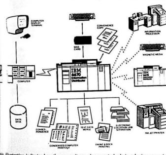
s illustration indicates how the new unit can play a central role in a business organiza-through its ability to access and process a wide variety of information. The IBM 6670 its with a laser, receives and transmits documents electronically, processes text and 0, and east. and can also make convenience copies
